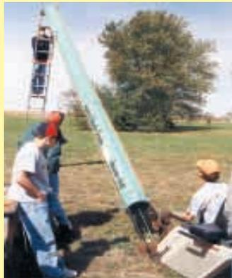
Pumpkin launcher works something like a sling shot, using a 20-ft. length of PVC pipe as a barrel. Exercise bike pulls pumpkin down for launching.
