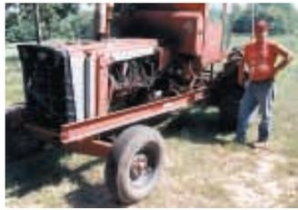
Tractor frame on back was reinforced with 6-in. channel iron.
