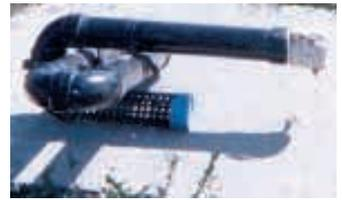
Oval-shaped water float is made up of four elbows and a couple pieces of 2-ft. long PVC pipe. Float holds intake nozzle about 4 in. from top of water and is perforated to keep screen from plugging up.
