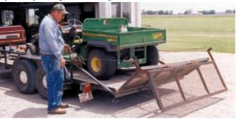
A winch-powered mechanism makes it easy for Richard Martin to fold and unfold the 5-ft. long ramp on back of his trailer.
