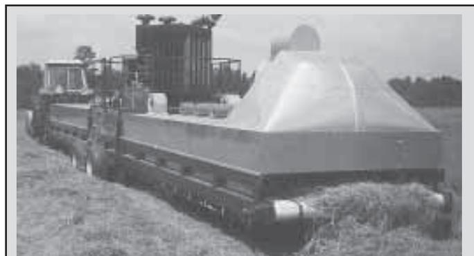
**Prototype microwave hay dryer used 210 household-type microwave units to dry high-moisture hay.**
