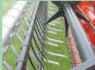
Out-front manifold puts nozzles down between reel fingers, ahead of knife.
