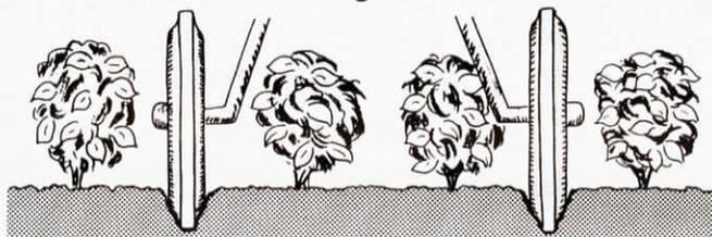
of two groove-making attachments, mounting brackets for both the planter and cultivator, and two single-rib front tires mounted on rims. In addition to all row-crop planters, the groove-making attachments can be mounted on Tye drills used for planting soybeans or other cultivated crops.
