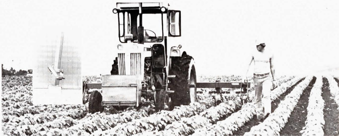
Although obviously not recommended as standard practice, Jack Larson walks beside "driverless" tractor to demonstrate Cultiguide guidance system. Tractor is equipped with single rib front tires which ride in grooves, as shown in drawing below.
