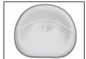
Farmall pan seat cushion has a steel core and a brass drain hole.
