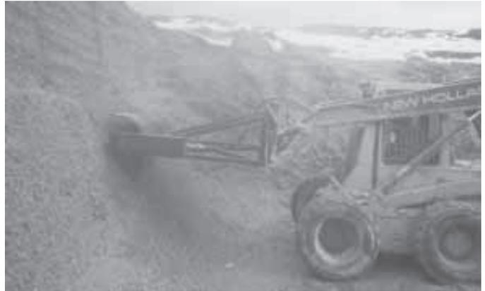
Silage defacer was custom-built for an older skid steer loader that didn't have enough hydraulic capacity to run most commercial units.
