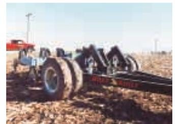
“Wille Built” caddy can be used to pull drills, planters, anhydrous toolbars, and subsoilers.
