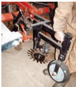
Trash-clearing wheels mount on independent frame fitted with its own gauge wheel.
