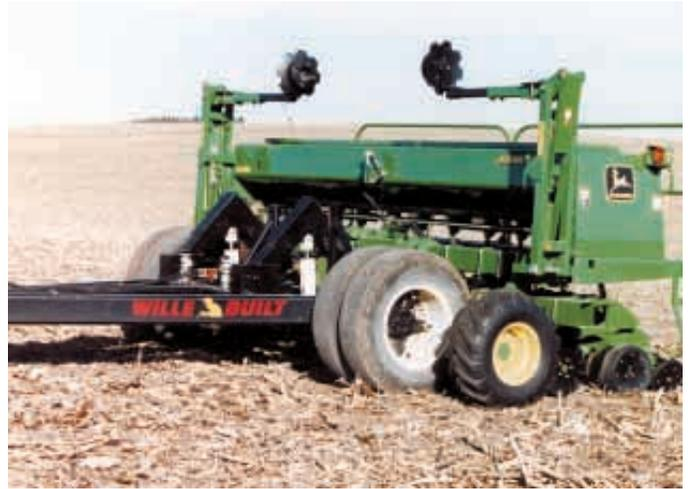
Semi-truck trailer axles fitted with dual wheels are used to build the heavy-duty caddy.
