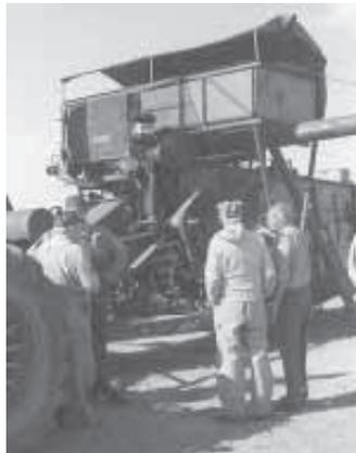
Machine's hopper and unloading auger is off an old Case pull-type combine. The hopper was enlarged by cutting the sidewalls away from three hoppers and then welding them together.
