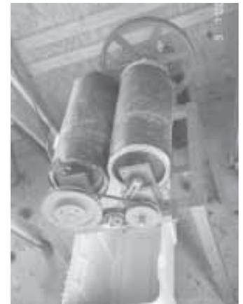
Home-built chestnut dehusser consists of two 3-ft. long, 8-in. dia. padded drums that rotate at slightly different speeds, providing the friction to rub off prickly husks.
