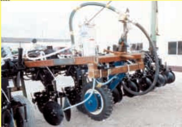
Planter toolbar is equipped with Yetter strip-till row units, as well as a GDI ground-driven pump and hoses that hook up to a trailing anhydrous ammonia trailer.
