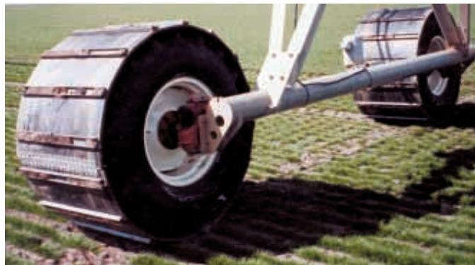
Fitted with metal traction bars, rubber tracks are designed to mount over dual wheels.
