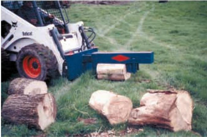
Vaaler splitter is equipped with a steel push plate on back. Plate moves forward to split log against a wedge that mounts up front.
