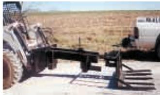
Optional "chunk scoop" quick-taches to front of splitter and allows you to load split chunks into a wagon or truck.
