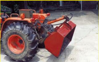
Being 75 plus years of age, I've now reached the point that it's time to use mechanical and other means substitute for muscle power. My 19 hp Kubota 4-WD tractor had dealer-installed hydraulics for lifting a snowblower. I simply rerouted the hoses so I could operate a custom-built, hydraulic dump bucket that mounts on the tractor's 3-pt
