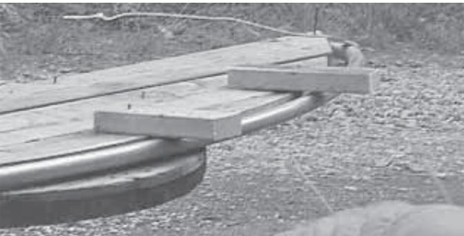
Three boards mount side by side on one end of spool, with several short blocks on top to keep tubing from slipping off as force is applied to bend it.
