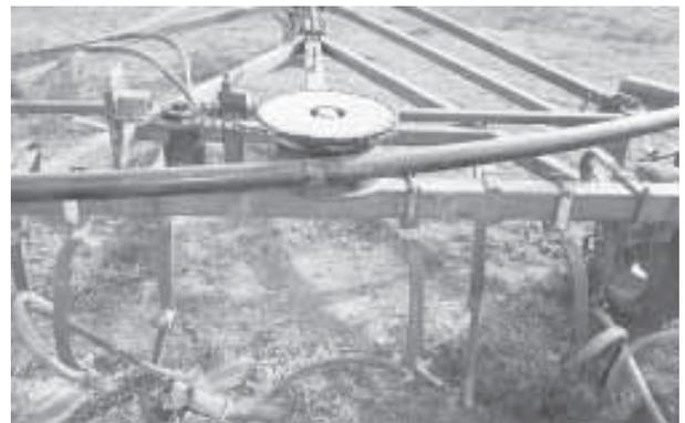
Wheel rims mount at the center of drill's middle section and on the end of the wings. As pipe is fed through, a hydraulic motor chain-drives the center wheel rim.
