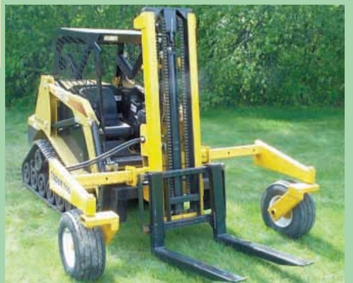
Two-wheeled mast attaches to skid steer loader arms. It uses a pair of hydraulic cylinders, and a chain-drive pulley system, to lift loads on a pair of 4-ft. forks.
