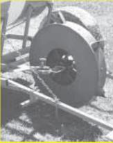
"Water wheel" planter has a 24-in. dia. steel wheel on back fitted with points that poke through plastic. Water is gravity-fed through a hose into open side of wheel.
