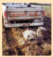
Leading edge of sled is placed against back side of rock. Then Langeland hooks chains around front side of rock and drives ahead until sled digs itself under rock.
