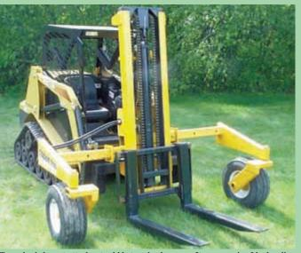
Two-wheeled mast attaches to skid steer loader arms. It uses a pair of hydraulic cylinders, and a chain-drive pulley system, to lift loads on a pair of 4-ft. forks.
