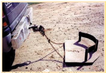
"Stone sled" is designed to skid along the ground behind a pickup or tractor.
