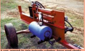
A ram, powered by twin hydraulic cylinders, forces wood chunks through stationary wedge.
