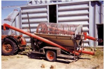
Seed cleaner measures 4 ft. in dia., 9 ft. long and is equipped with a pair of augers for Both augers fold up alongside drum for transport. loading and unloading.
