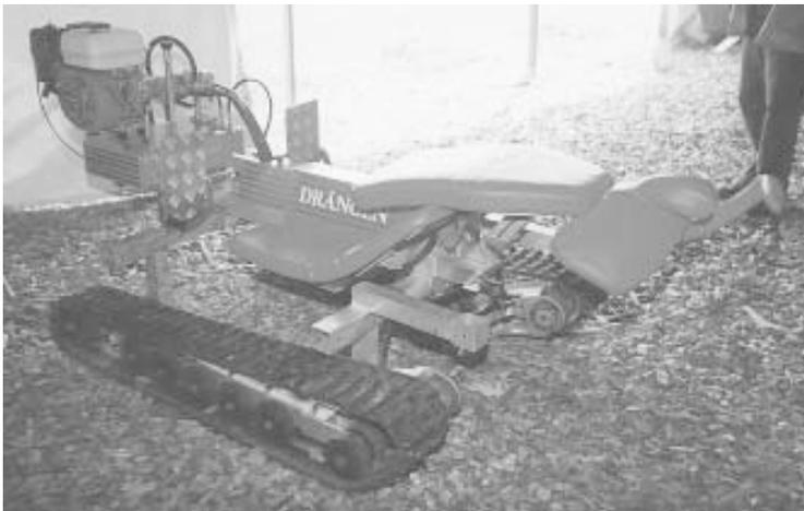
Motorized laydown work cart looks like a massage table mounted on snowmobile treads.
