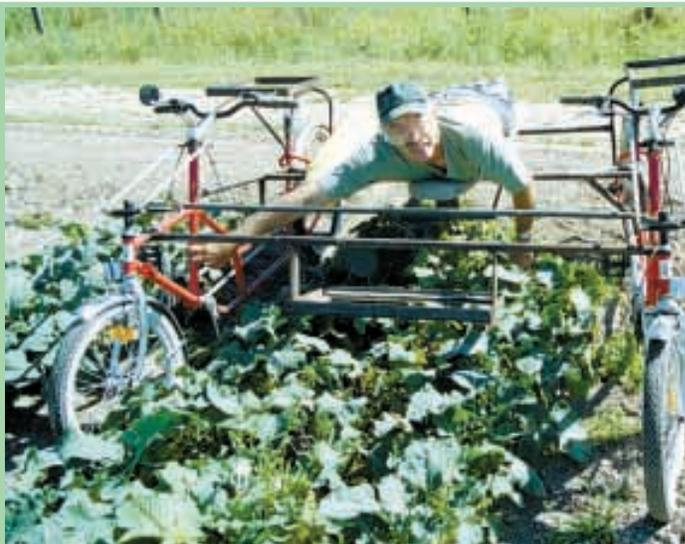
Glen Johnson built this wheeled machine to straddle his 3-row, 48-in. wide vegetable beds. The worker lies on a padded board that can be adjusted from side to side across the frame to make it easier to reach all of the planting bed.
