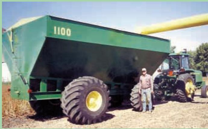
**Big 4-wheeled pull-type cart holds 1,100 bu. of grain and has a front-mounted, turret-style auger that can load a semi from either side of cart.**
