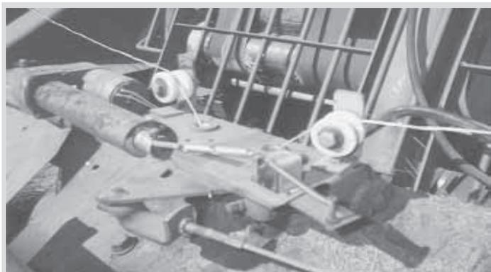
A pair of electric fence insulators mount on front of Egli's New Idea 484 baler. Twine travels over insulators, turning them, so he can see whether the twine is moving.
