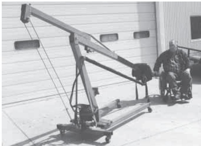
Don Skinner modified this stationary lift boom, adding a 4-ft. length of steel tubing behind the lift arm and mounting a seat on the end of machine's telescoping lift arm.
