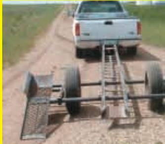
ends about 6 in. above the ground. Each saddle and ramp is welded to a short length of steel pipe that rides over a smaller pipe. To load the trailer, I drop the ramps down to the ground. I drive the Spra Coupe's single front wheel up onto the runway and then slowly drive the rear wheels up the ramps and into the saddles. As the saddles drop down, the ramps automatically tip up ready for transport.
