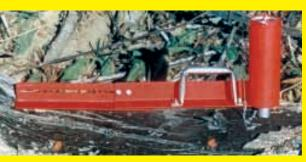
Here's a new idea I call a Firewood Measure Marker. It's adjustable from 14 to 26 in. long and helps cut firewood to uniform lengths, which makes stacking and storing easier. With a slight touch it leaves a small spot of paint on the wood so you know where to make the next cut. We've made up a prototype and the tool is
