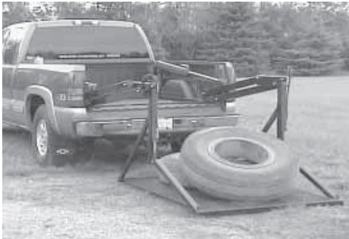
Remote-control lift platform handles loads up to 1,000 lbs.
