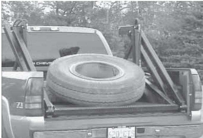
Platform stays level as it lifts load from ground into pickup bed.
