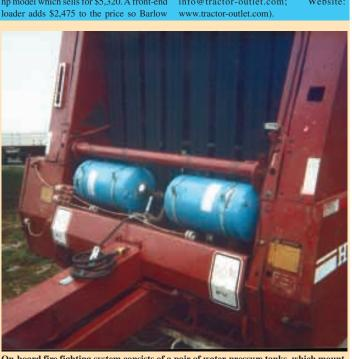
On-board fire fighting system consists of a pair of water pressure tanks, which mount in an open area above the hitch. A 10-ft. length of 3/4-in. hose is used to put out fires.
