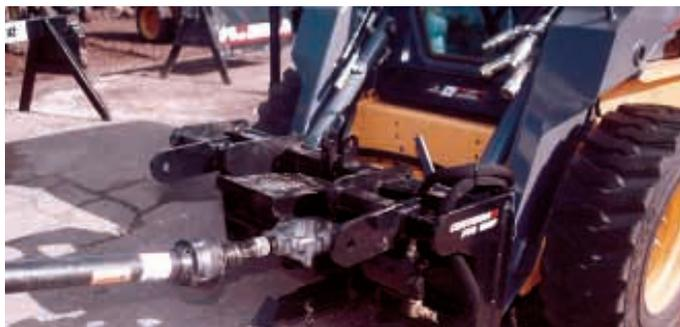
Hydraulic-powered pto adapter gives you the choice of using either hydraulic or pto power with your skid loader to operate a wide variety of attachments.
