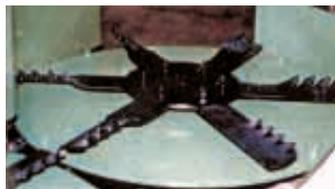
**Rotto Chip blades bolt onto existing chaff spreaders in place of original deflectors. A series of upward-pointed teeth on blades are used to "chip" weed seeds.**
