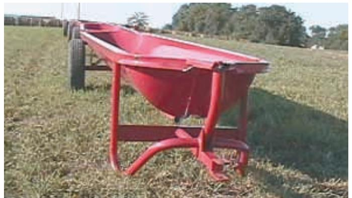
Special hitch on front bunk hooks to tow vehicle.
