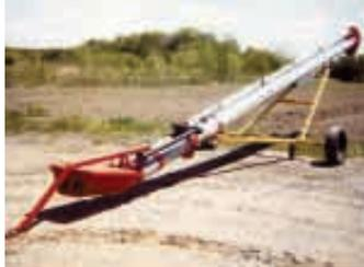
Everett Meister bought a used 60-ft. 8-in. dia. auger, cut it in half, and then put the two halves together.
