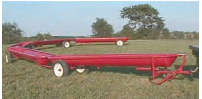
As many as 10 feed bunks can be hooked together to tow behind a tractor or pickup. All-steel bunks measure 12 ft. long, 26 in. wide, and 12 in. deep.
