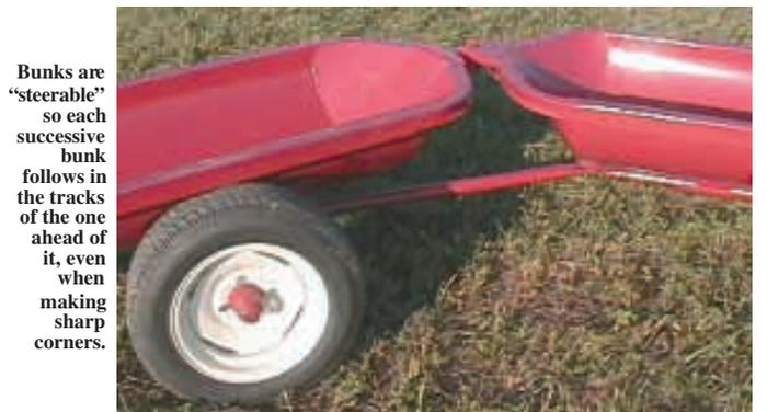
Bunks are "steerable" so each successive bunk follows in the tracks of the one ahead of it, even when making sharp corners.
