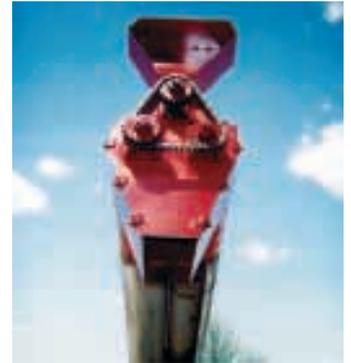
Two short lengths of auger flighting deliver grain from home-built metal hopper to twin augers. Driveshaft runs from pto shaft up to three drive sprockets.
