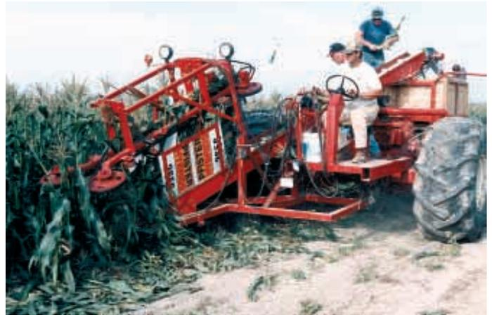
Hydraulic-driven machine grabs stalks high up between counter-rotating rubber belts and pulls them back through a pair of rollers that pinch ear off stalk.
