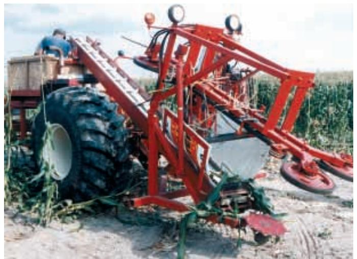
Ears fall onto a conveyor which drops them into a large wooden hopper on back of machine. Rotating steel disc in front of conveyor cuts stalk off near ground.
