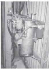
He made a power pack for the elevator from a 110-volt electric motor and a 2speed hydraulic pump.
