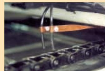
Continuous oiling reduces friction to prolong life of machine.
