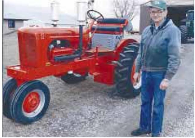
The Litchfields fitted an old Allis Chalmers WC tractor with a Chevrolet 283 V-6 engine and mounted a Mig welder under an extra wide seat.
