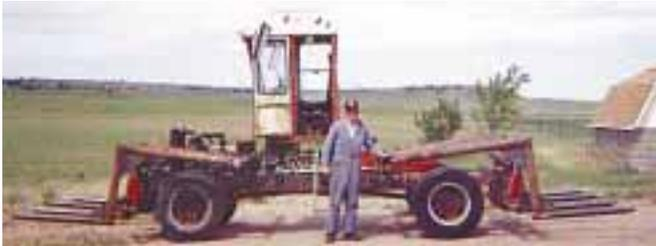
Unit has two separate sets of forks on each end mounted on L-shaped loader arms.
