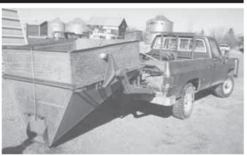
Hagg used a 1930's Case combine grain tank to make this pickup-mounted feeder. It's raised and lowered by bale-handling arms on his 3/4-ton pickup.
