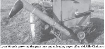
pull-type combine into a 3-pt. mounted, hydraulic-driven feed hopper.
