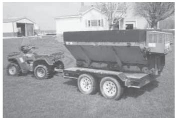
Roberts mounted road sander on a tandem axle trailer. Rear-mounted gas engine is used to drive an auger that runs down middle of road sander and empties out the back.
