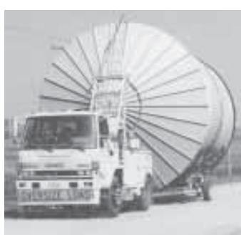
**Bins can be lowered to a horizontal position on a trailer.**
