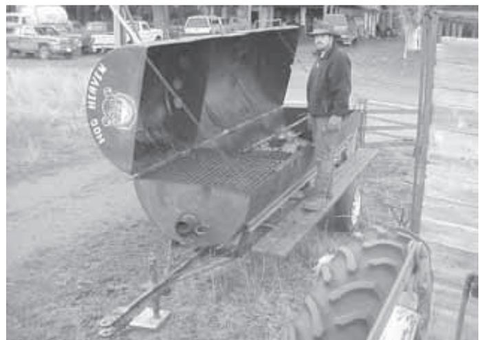
Bill White built this whole hog cooker out of a 2,000-gal. diesel storage tank. One half is used as an open barbecue and the other as an oven-type cooker.
