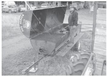
Bill White built this whole hog cooker out of a 2,000-gal. diesel storage tank. One half is used as an open barbeque and the other as an oven-type cooker.
