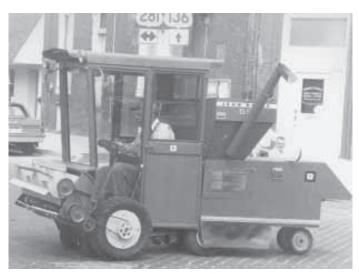
Pritts built this scale model Deere 55 combine on a Snapper riding mower. It has a cab, platform head, grain tank, working augers, and straw chopper. an 11 hp Honda engine.
