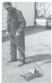
To pick up a log, Kindig twists the handle clockwise with his right hand, which rotates a single tong sideways toward two stationary tongs.
