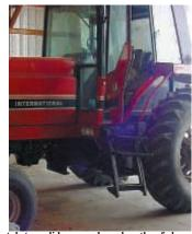
Powered by an electric winch, expanded metal steps slide up or down lengths of chan-nel iron that bolt to tractor frame. Winch is operated by a simple up-and-down control switch that mounts on cab door.
