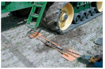
Sensor consists of a fluid-filled 1-in. dia. rubber bulb attached to a pressure transducer by a high-pressure hose. Specially-designed drill bit is used to insert bulb into soil.
