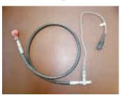
Pressure on bulb is read by either an electronic sensor or a simple dial pressure
