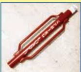
Unit has a spring-loaded plate that strikes post. After it hits, the compressed spring bounces the driver back up for the next blow.
