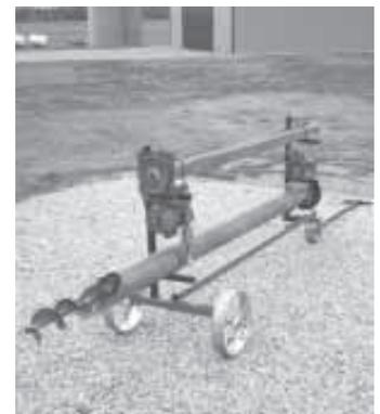
Mike Grace's home-built “auger caddy” carries a 6-in. bin unloading auger as well as a sweep auger.
