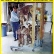
held by wooden racks bolted to a pair of vertical wood posts, which are in turn bolted at the bottom to a steel frame. The frame rides on four castor wheels and is widened out on front for added stability. To steer the caddy, I hold onto a length of pipe that's connected to the frame. It steers much like a tiller steers a boat. (Mark Kimes, Beecher City, III.)
