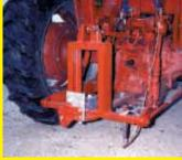
the pintle hitch to the plate. I spot welded nuts for 1/2-in. bolts on the back side of the plate. There are three sets of holes so six nuts were required. And four bolts were needed to mount the pintle hook. In addition, two 3/4 by 6-in. grade 8 bolts were used to attach the bracket to the drawbar frame. The addition of a spacer allows the pintle hook bracket to set squarely to the drawbar. Then 3/4-in. nuts were spot welded in place on the top side of the 2 by 3 tubing.
