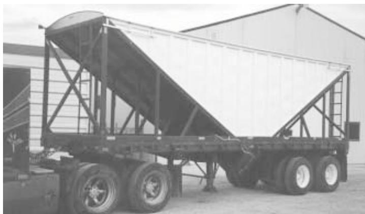
Van Kemenade and Lindsay bought a used 28-ft. flat deck trailer and mounted a double compartment hopper on it that they built from scratch.
