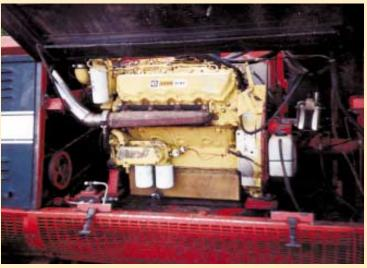
Pat Minehan found out that repairing or replacing the 540 Perkins diesel engine in his Massey Ferguson combine would have been too expensive. He decided to "upgrade" to a Caterpillar 3208 diesel that came out of a New Holland TR70 combine..
