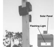
Solar-powered unit uses red flashing light to scare away predators. One light will protect about an acre. Photo shows four units mounted on one pole.
