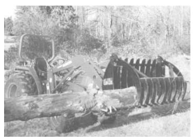
Grapple rake uses a hydraulic-operated grapple to clamp and hold material. "They're ideal for loading logs, picking up rocks, and piling brush," says Anbo Mfg.
