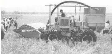
"Mini stripper" consists of a custom-built, 8-ft. Shelbourne Reynolds stripper header mounted on an articulated, 4-WD Case ditcher.
