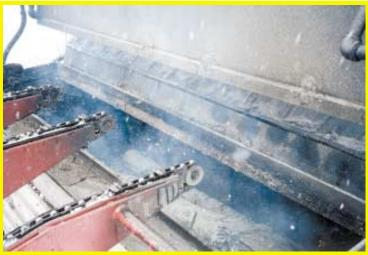
Firebox is big enough to handle 8-ft. logs, which are automatically fed into furnace by a modified Farmhand stack mover that's hydraulic-powered and handles up to 3 cords of wood at a time.
