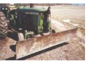
Blade is held to tractor by a pair of 4-in. dia. pipes that run back to rear axle. An 8-in. cylinder raises the blade.
