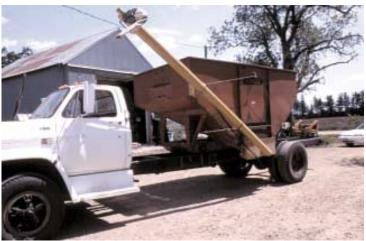
An orbit motor at top of auger plugs into outlets on tractor that Reed uses to pull his grain drill.
