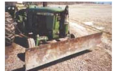
Blade is held to tractor by a pair of 4-in. dia. pipes that run back to rear axle. An 8-in. cylinder raises the blade.
