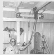
Each hoist carrier is fitted with two 12-in. railroad wheels.
