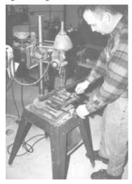
and bolted it to the base of a drill press. The cross slide has its own small vise for hold-
