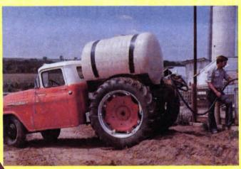
Being half tractor and half truck, the Truck-Tor is tailormade for highway use (it travels up to 50 mph) and has reversible pto for use around farm as a second tractor.
