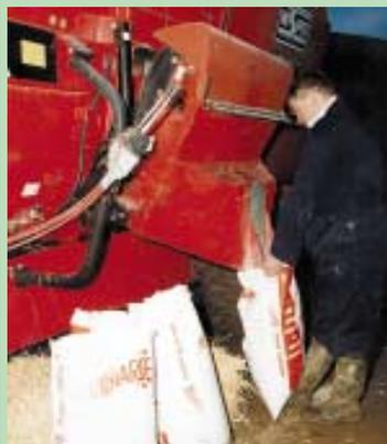
Graham Band turned a side-unload feed wagon into a handy "bagger" by adding a home-built bagging chute to the side of the unit.
