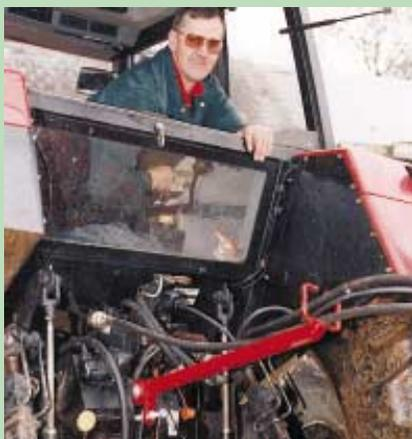
Steel bracket attaches to 3-pt.'s top link to keep hoses in place.
