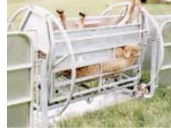
To tip the animal you simply rotate one of the large wheels at each end of crate.
