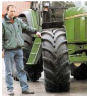
Lugs on Vredestein tire are closer together at center and farther apart at outer edges.
