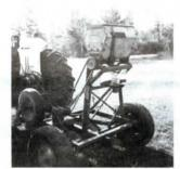
tic mounted ahead of the fan deflects seed that's thrown forward. To change seeding rates I simply adjust the opening on the box. I pull a 6-section harrow behind the seeder to cover the seed and to make a mark for the next round.
