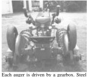
cones on front of the augers help the tractor climb over sidewalks and tree roots, etc. The tractor has a Chevrolet 3-speed transmission that's connected to an Avery transmission by a short driveshaft. A single tire in front, and a pair of spare donut car tires on back, can be lowered to the ground in order to raise the augers and keep them from gouging into the ground.
