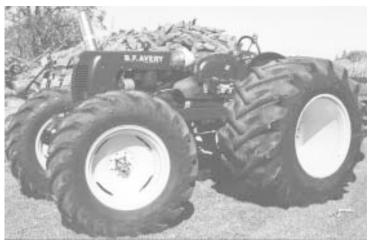
**4-WD "Big Foot" -** "Everyone wants to see me drive this one," says Melton. It's a 1946 Avery equipped with a Jeep front axle and four huge combine tires - 30.5 by 32's on back and 14.9 by 26's on front. A 4-cyl. Hercules turbocharged engine supplies the power and is connected to the tractor's
