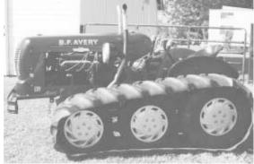
Full Track - This 1946 Avery rides on a pair of 18-in. wide, 38-in. long rubber tracks made from two rear tractor tires off a Deere 4340 tractor. The tracks are supported by three sets of axles. The center and front axles are rear axles off Oldsmobile Cutlass front wheel drive cars. The rear axle is original
