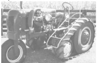
Half Track - This 1946 Avery is equipped with 15-in. wide, 38-in. long "half tracks" and a single 16-in. front wheel. The track was made by cutting up tractor tires. It's powered by a V-6 turbocharged engine off a Buick Regal car and also has the car's automatic transmission. The track is supported by 22-in. tires on back and 14-in. tires up front. The axle that connects the front tires pivots to
